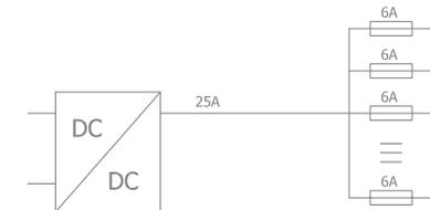
A distribution system using power supplies or DC-DC converters without "battery fuse".
