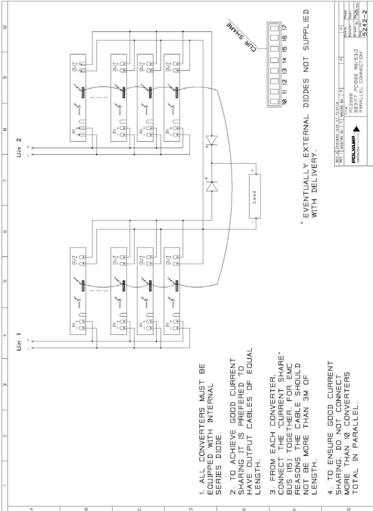
Figure 9. Two supply systems with common load and parallel converter outputs.
