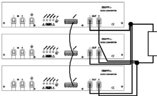
**Figure 3. Current share connection with series diode.**
