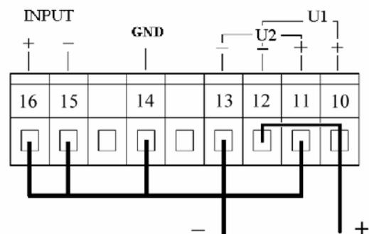
Figure 4. Output "U1" to output "U2" isolation test
