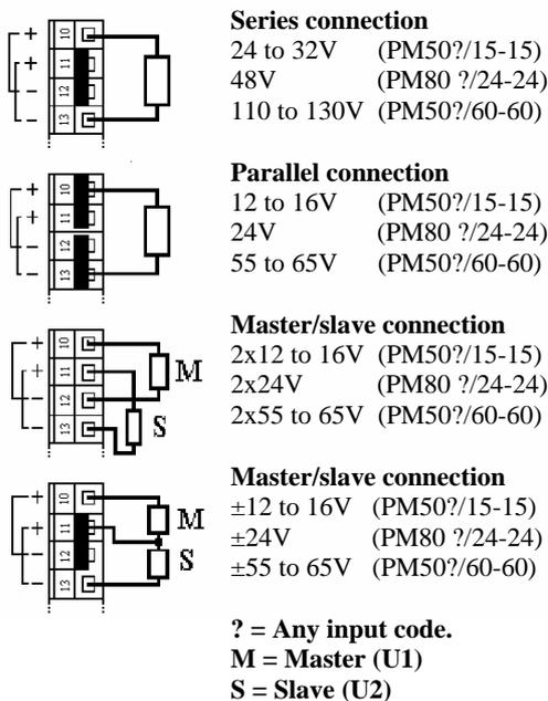
**Figure 1. Output connections**
