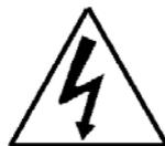
The lightning flash with arrowhead, within an equilateral triangle, is intended to alert the user to presence of uninsulated "dangerous voltage" within the products enclosure that may be of sufficient magnitude to constitute a risk of electric shock to persons
