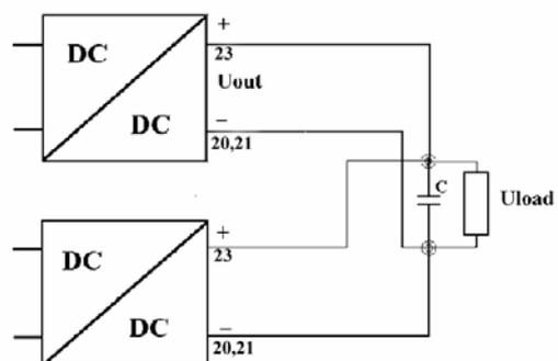
**Figure 2.** Voltage drop  $U_d = U_{out} - U_{load}$
