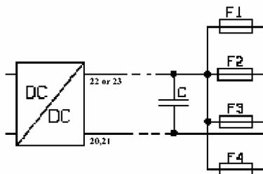
Figure 5. Connecting multiple loads.
