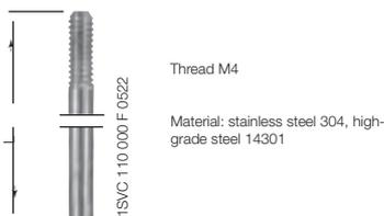
During project engineering the compatibility of the electrode material with the medium to be supervised is to be examined!
